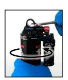
91. Use a strap wrench to grip the air can while using a torque wrench with a 13 mm crowfoot socket to tighten the air can eyelet to 16.9 N·m (150 in-lb).
