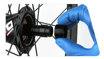
Install the driver body onto the axle and twist it counter-clockwise to seat the driver body and driver body seal.
