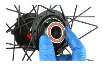
Slide a SRAM 63803 bearing press tool onto the threaded rod of the Wheels Manufacturing® Press-1 Sealed Bearing Press tool. Insert the threaded rod of the bearing press through the non-drive side of the hub shell. Slide the SRAM 6903 Bearing Press tool onto the threaded rod.
