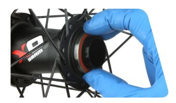
Slide a SRAM Bearing Press 23327 tool onto the threaded rod of the Wheels Manufacturing\* Press-1 Sealed Bearing Press tool. Insert the threaded rod of the Sealed Bearing Press tool through the non-drive side of the hub shell. Slide the second SRAM Bearing Press 23327 tool onto the threaded rod.
