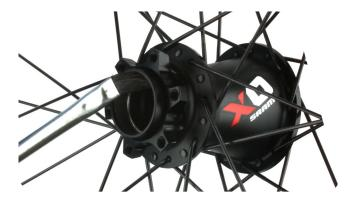
Install a new bearing into the drive side of the hub with the red seal facing outward.
