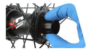
Install a new bearing onto the drive side end of the axle with the red seal facing outward.
