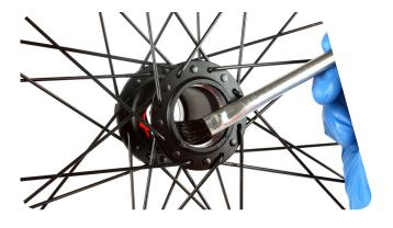
2 Install a new bearing into the non-drive side of the hub with the red seal facing outward.
