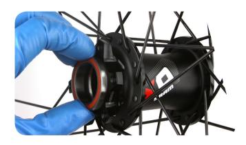
Slide a SRAM Bearing Press 23327 tool onto the threaded rod of the Wheels Manufacturing\* Press-1 Sealed Bearing Press tool. Insert the threaded rod of the Sealed Bearing Press tool through the drive side of the hub shell. Slide the second SRAM Bearing Press 23327 tool onto the threaded rod.
