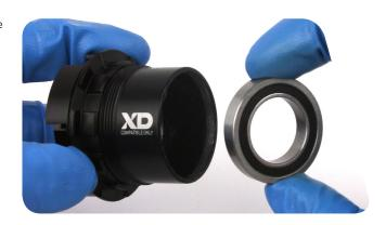
Slide a Wheels Manufacturing® 6804 adapter onto the threaded rod of the Wheels Manufacturing Press-1 Sealed Bearing Press tool. Insert the threaded rod of the bearing press through the non-drive side of the driver body. Slide the SRAM 63803 Bearing Press tool onto the threaded rod.
