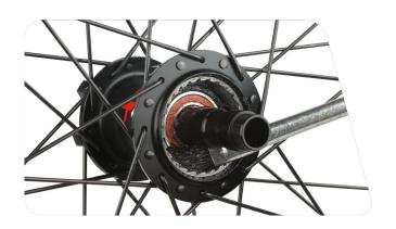
Use your fingers to install the spacer tube onto the axle.
