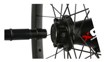
Install a new bearing over the axle and into the non-drive side of the hub with the red seal facing outward.
