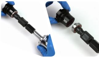
Use your fingers to remove the ID (inside diameter) spacer tube and the OD (outside diameter) spacer tube.
