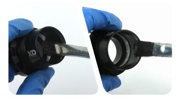
2 Install a new bearing into the drive side of the driver body with the **black** seal facing outward.
