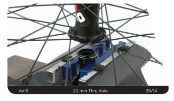
Use a soft face mallet to tap out the axle and bearing. Remove the bearing from the axle.
