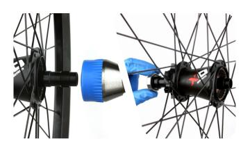
Insert the non-drive side of the axle through the non-drive side of the hub.
