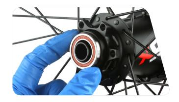
Slide a SRAM 6903 bearing press tool onto the threaded rod of the Wheels Manufacturing\* Press-1 Sealed Bearing Press tool. Insert the threaded rod of the bearing press through the drive side of the hub shell. Slide the second SRAM 63803 Bearing Press tool onto the threaded rod.
