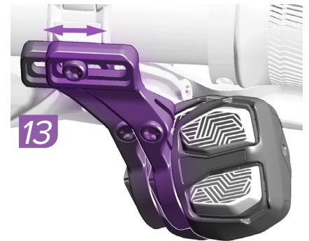
13. Move the bridge horizontally to the desired position.
