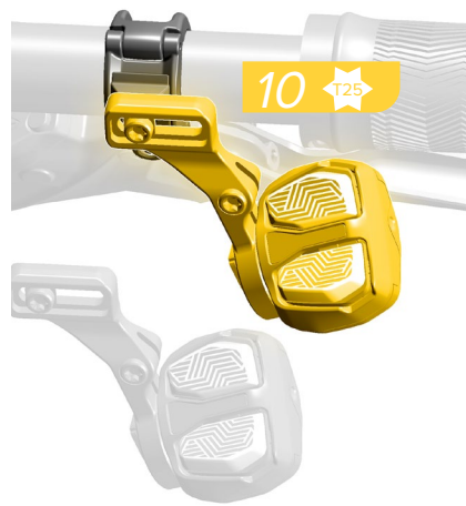
10. Install the bridge.
