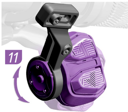
11. Rotate the controller to the desired angle.
