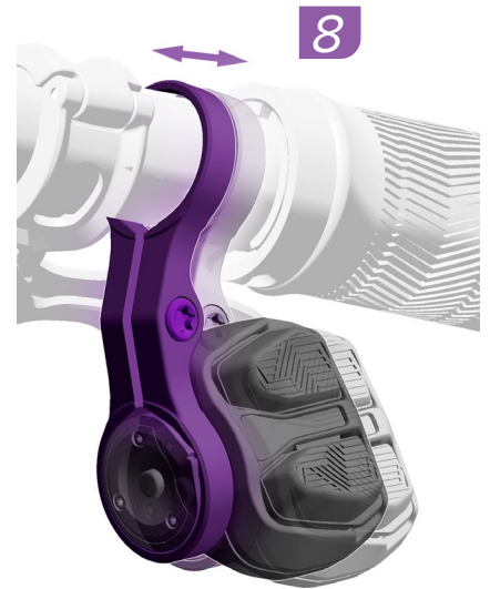
8. Move the clamp horizontally to the desired position on the handlebar.
