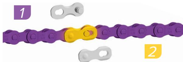
Pull each end of the chain together and install the PowerLink.
