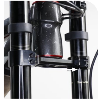
Upper Tube / Crown Height Gradient Position - Spring Side
