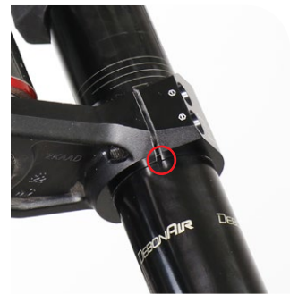
Incorrect - Not within lower crown gradient
