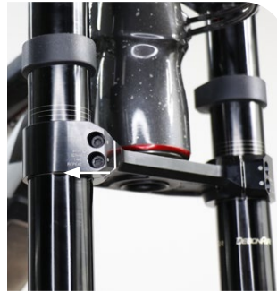
Upper Tube / Crown Height Gradient Position - Damper Side
