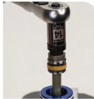
Piston tool and 14 mm socket
