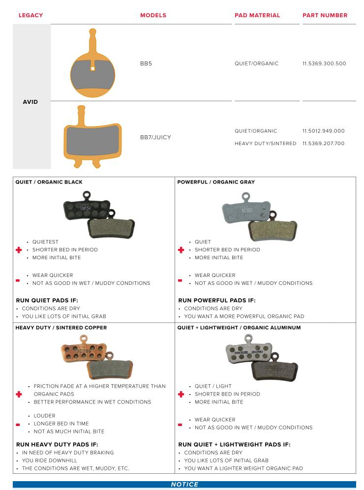
Changing pad material: When changing disc brake pads, if the new pads are of a different material than the currently installed pads, new rotors should be installed and a rotor 'bed-in' process should be performed. Consult the *Disc Bed-in Procedure* in the *MTB Disc Brakes and Shifters User Manual*, the *eTap AXS Systems Manual*, or the *HRD Shift-Brake Lever & Caliper User Manual*, available at <u>www.sram.com/service</u>.
